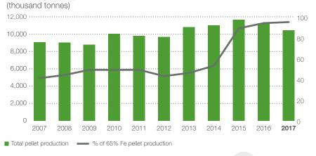
In 2015, the Group completed its **Quality Upgrade Programme** to increase the iron content of its pellets to 65% Fe. As such, production of 65% Fe pellets has increased from 53% of total output in 2014 to 95% of total output in 2017, a record for the Group.
