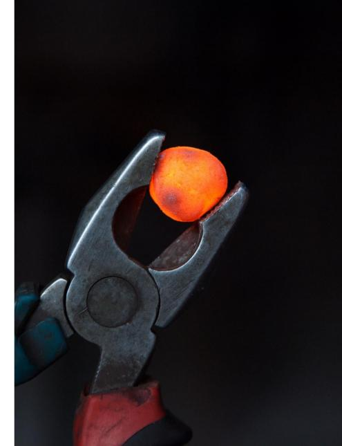
Image: an iron ore pellet immediately after exiting the Group's pelletiser, which heats concentrate to over 1,300°C using a combination of natural gas and biofuels (sunflower husks).
